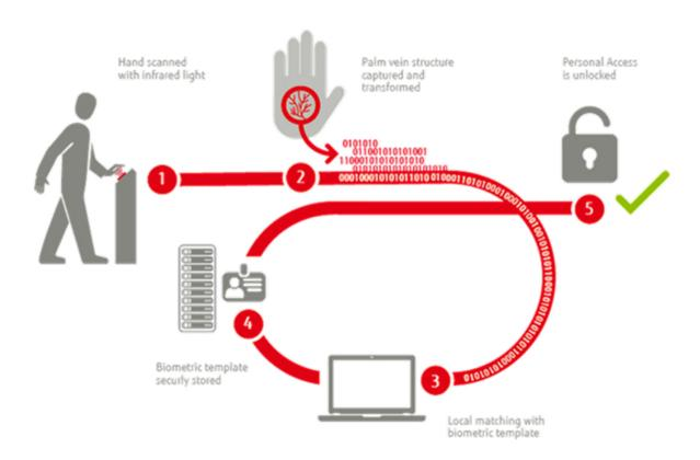
When a person places their hand above the PalmSecure sensor, it emits a near-infrared light that records the palm vein pattern and the sensor encrypts the received data. The encrypted data is transferred to the PC, and the software converts it to a biometric template and assigns it an individual key.
